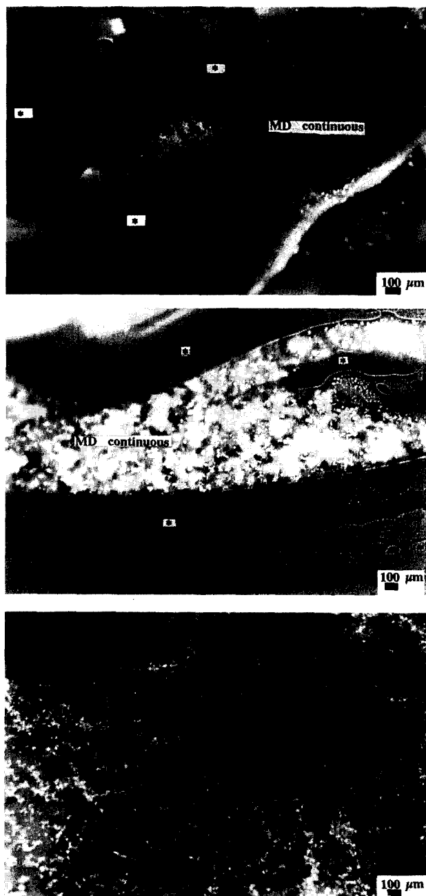
Fig. 6. Bright-field-optics micrographs of 5% gelatin with 12% maltodextrin taken at 60, 30, and 20 °C (top, middle, and bottom images, respectively). In the top two micrographs, (*) indicates the gelatin phase. Details of sample handling are given in the Methods part of the paper.
